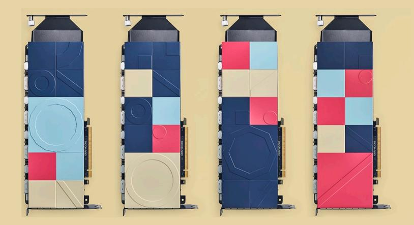
DOUBLE WIDTH PCIE CARD WITH 2 – COLOSSUS GC2 IPU PROCESSORS CARD-TO-CARD IPU-LINKS<sup>™</sup> (320GB/s) 250 TERA-FLOP MIXED PRECISION IPU COMPUTE @ 300W
